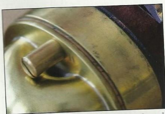
This shows a close-up of a bassoon's cork on the U-tube that is in excellent condition. If it does not look like this, replace it.
