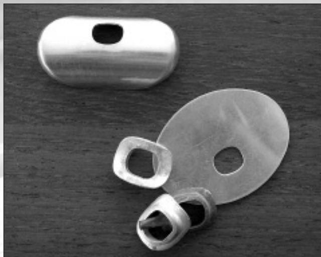
Risers are cast like pieces of jewelry, ready to solder under the lip plates. Lip plates are shown here fresh from the stamping dies.
