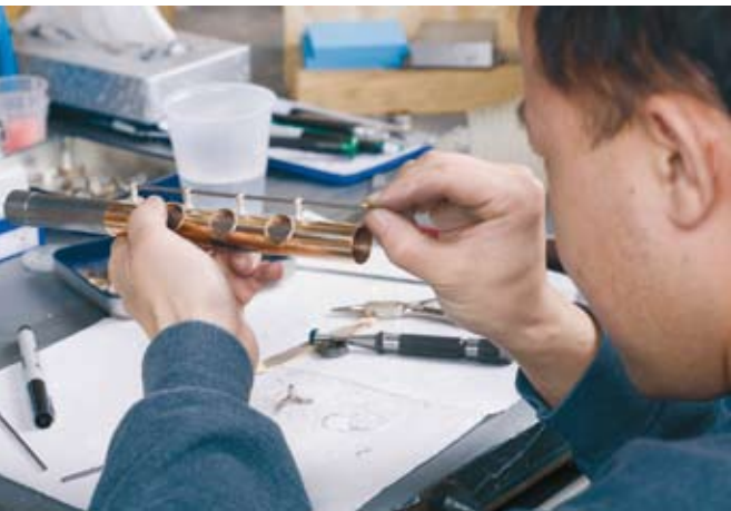
Checking the alignment of the pillars.
