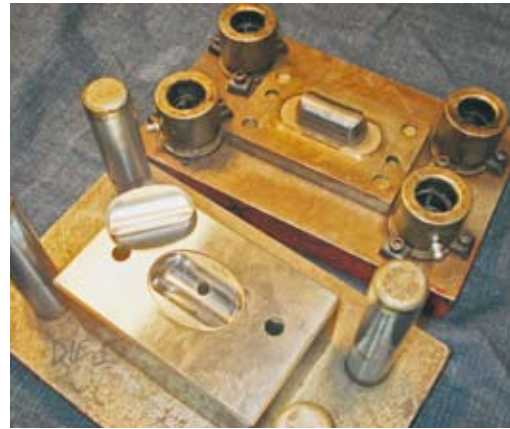
The top and bottom halves of the press tool that stamps out lip-plates.
