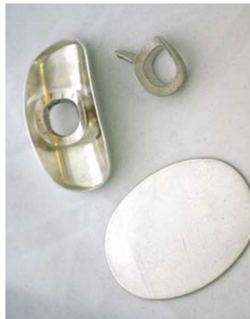
Lip-plate parts: A complete lip-plate, a silver casting for the riser and a silver blank ready to be stamped into a lip-plate.
